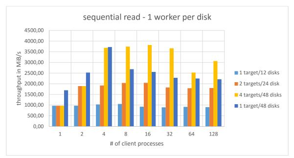
For the tests with 1, 2, and 4 individual RAID6 targets we see that the performance peaks between 8 and 32 processes to a maximum – and reduces a bit when going to 64 and 128 processes due to the higher number of concurrent accesses to the same amount of disk drives
