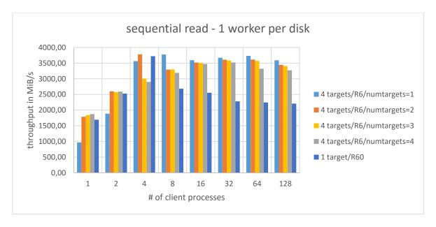
For 1 and 2 client processes any numtargets setting larger than 1 can exceed the performance of the RAID60 target. For 4 client processes a setting of 3 and 4 for numtargets falls behind the RAID60-configuration. For all larger process counts a setting of 1 on the setup with 4 individual targets gives the best result – and the RAID60 configuration is significantly worse.
