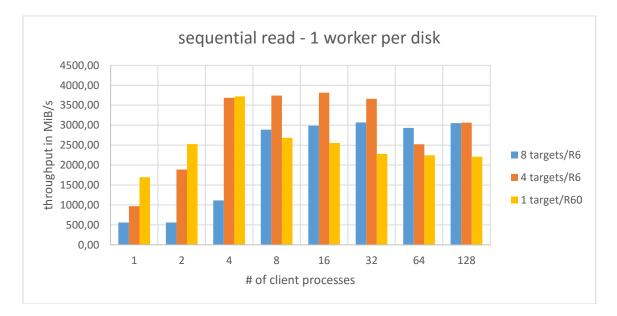
When doing sequential reads we see a significant difference in performance with the 8-target configuration – just for 64 processes we see a slight advantage – and for 128 processes a draw with the 4-target configuration. For all other tests the new configuration performs worse. Especially with a low process count (1, 2, 4) it has a disadvantage as the individual targets are much slower than before.
