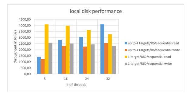
For the test with "up to 4 targets" 8 threads work on a single target, 16 threads work on 2 targets (8 assigned per target) etc.
